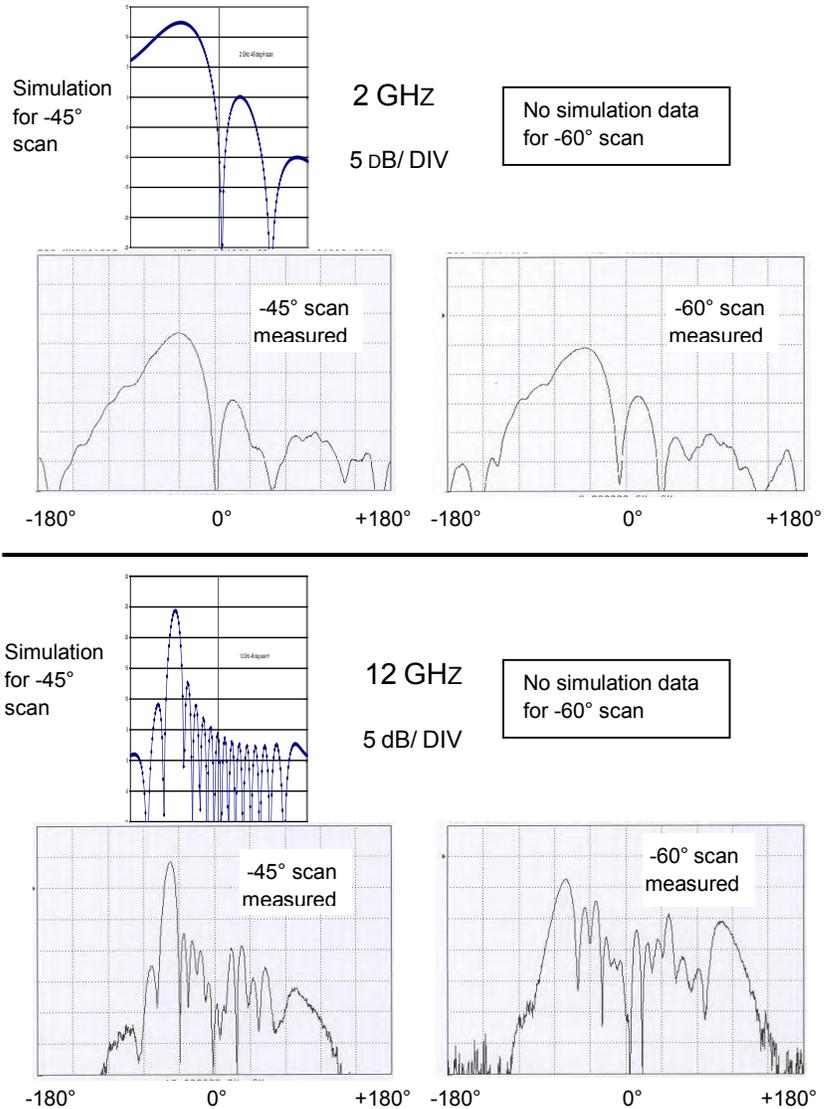
Fig. 5. Comparison of measured and simulated radiation patterns of prototype array for -45° and -60° scan at 2 GHz and 12 GHz.
