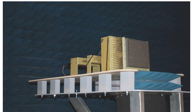
Fig. 3. Far-field measurement of the prototype array with banks of BSN in anechoic chamber.
