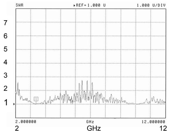
Fig. 4. Measured SWR for array with 0° scan.
